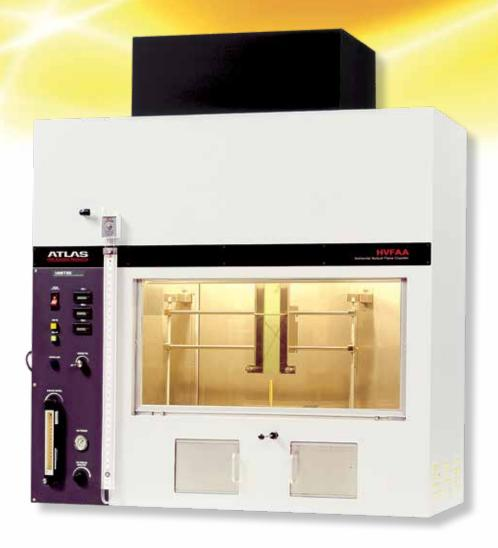
Atlas' HVFAA Horizontal Vertical Flame Chamber accurately determines the flammability of cabin compartment materials and electric wire. The chamber is designed to perform Bunsen burner tests in accordance with FAA's *Aircraft Material Fire Test Handbook* DOT/ FAA/AR-00/12, chapters 1.0 - 4.0 (FAR 25.853, 25.855, 25.1359).
