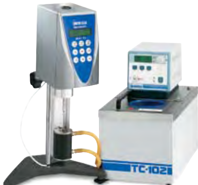
TC-102 Water Bath (p29) Small Sample Adapter (p32) SC4-27 Spindle (p42) SC4-13RPY Sample Chamber w/RTD probe (p42)
